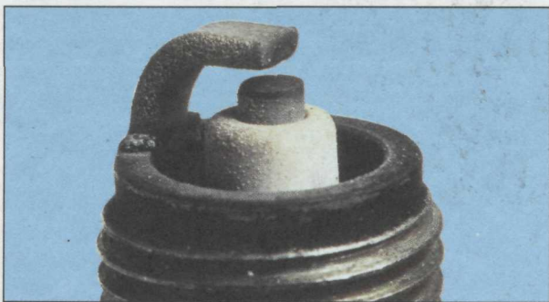
Normal condition – A brown, tan or grey firing end indicates that the engine is in good condition and that the plug type is correct.
